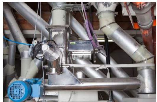
Blending optimization with NIR-Online Process Analyzer and bypass sampler.
