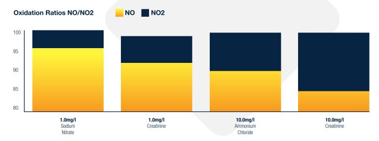
The unique features of the chemiluminescence detector gives The Sercon Thermalox TN analyser its remarkable sensitivity, at least an order of magnitude more than other available systems, by calibration, TNb is determined from the amount of NO measured.
