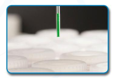
The  $\mu L$  Workstation uses encoder feedback to ensure accurate and precise location, enabling the use of microtiter plates up to 384 wells.
